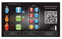
button until bottle counter flashes on display and two beeps are heard. Bottle counter will reset to zero once you release dispense button. Exit maintenance mode by tapping dispense 5 times in 10 seconds.
