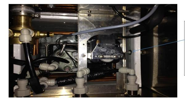
This is the Overflow Outlet inside the Machine Unit – Add enough water so the water level is just a little under the overflow outlet
