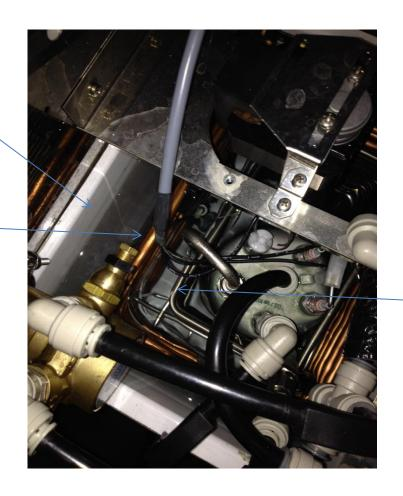
Stainless Steel Pipes – CAN NOT BE FROZEN – If there is ice – DO NOT USE MACHINE – Turn off – wait for ice to melt
