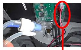
8. Unclip the White, Red and Black wire connectors from PCB to allow Front Cover to be removed.
