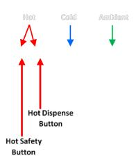
The above picture shows the Front Water Dispense Buttons for the *Waterlogic WL270 Water Treatment System*.
