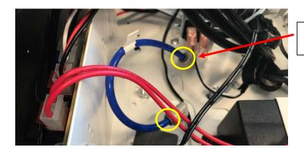
DISCONNECT TO BREAK THE VACCUUM AND ALLOW WATER TO DRAIN FROM COLD TANK.
