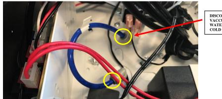
DISCONNECT TO BREAK THE VACCUUM AND ALLOW WATER TO DRAIN FROM COLD TANK.
