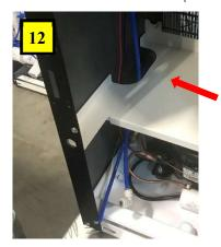
Drain port is located beneath shelf shown in photo.
