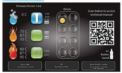
Enter maintenance screen by selecting ambient and tapping dispense 5 times in 5 seconds.
